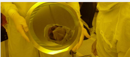
Markus Wimlinger shows Françoise von Trapp a 300mm bonded wafer on tape carrier.
