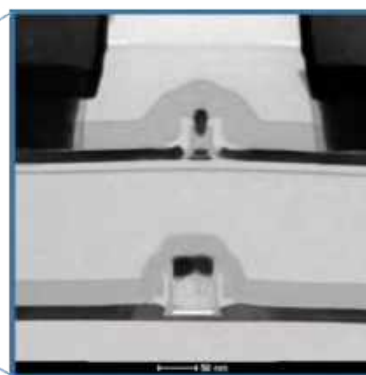
Figure 1: CoolCube™, CEA-Leti's version of 3D sequential integration allows device stacking at nanometer-scale resolutions, allowing for low aspect ratio and small 3D-contact fine-grain interconnects.
