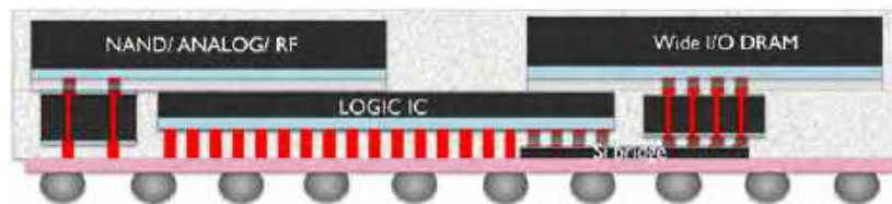
Figure 1: Concept of the flip-chip on fan-out wafer-level package.
