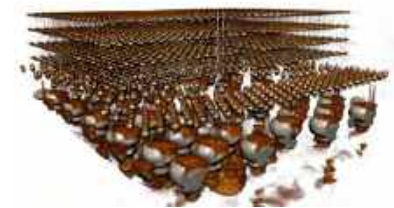
Figure 5: 3D rendering of all the internal interconnects extracted from Versa XRM 3D dataset showing the hierarchy and complexity of package interconnect.
