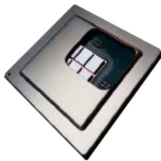
Figures 2a and b: A 3D multicore circuit called IntAct is said to offer five times more processing power and double the energy efficiency of the best 3D circuits currently available.
