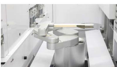
Figure 3: High-speed wafer transfer via the Trymax equipment front-end module.
