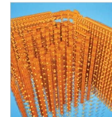
Visualize structures and defects within intact 15-die DRAM package
